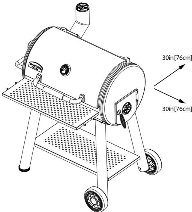
30in[76cm] minimum clearance from any combustible surfaces
